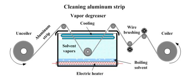
Coils of clean aluminum strip are transferred to the cladding line.
