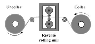
The strip of aluminum alloy clad with pure aluminum is then cold rolled to the final thickness for several rolling passes prior to bonding with steel back.
